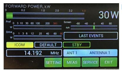
Measured driving power is 30 Watts.
