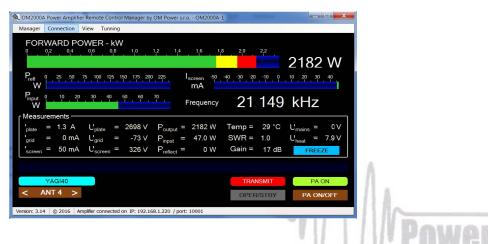
Fine tune screen: It is possible to retune the PA TUNE and LOAD remotely (See page 31).
