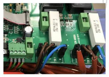
There are AC selector for each transformer. The blue wire – one side of primary winding is conected to N pole. Wire marked with proper voltage connect to L pole.
