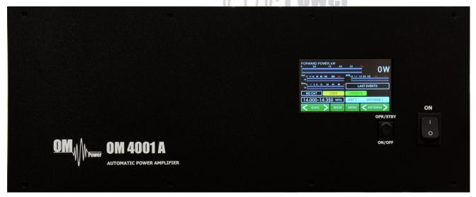
**ON** - **Main Switch.** After turning ON, a small 12V APU for logic, protection circuits and the display will be activated. High voltage and RF circuits are still OFF.
