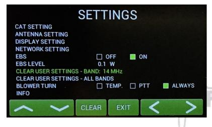
The next two settings allow deletion of the manual user settings of the amplifier tunings for a single band or for all bands.
