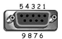
RS232 connection to the computer. For CAT communication connect pin 2 TX-D, pin 3 RX-D and pin 5 GROUND
