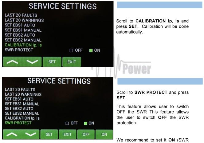
protection circuit will stay active, max. allowed SWR is 3:1). If **OFF** is selected, higher SWR is allowed, but reflected power is measured. If it exceeds 350W, transmit will be blocked.
