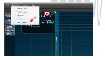
Now connect the USB-FTDI adapter to a USB port on the Flex radio. A new line showing the connected USB adapter will appear.
