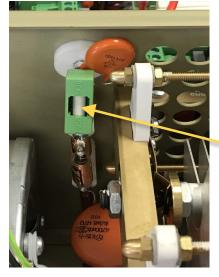
One special fuse, filled with sand, is used in the model OM40001A. In the case of an accidental discharges or short within the tube this fuse (4 Amps fast, filled with sand) saves the HV supply circuits.
