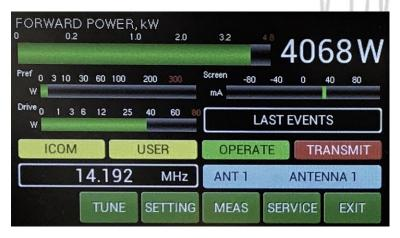
We can now see a new small yellow **USER** window in the touch screen display. **USER** means that we used the M-TUNE feature to optimize the PA adjustment.
