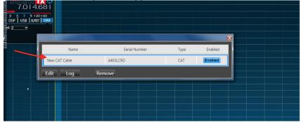
Double click on the new usb adapter line to open the configuration window for this COM port .
