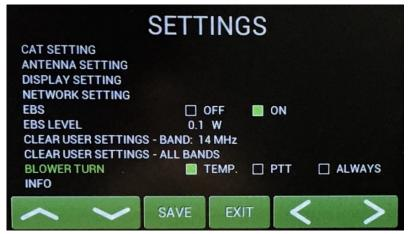
In the next line you can define working mode of the blower. In the first mode speed depends on the PA temperature (TEMP), In PTT mode the speed increases to maximum, and the ALLWAYS mode means maximum speed all the time PA during operation (recommended DIGI for modes).
